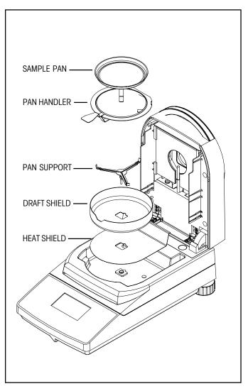
Open the cover and remove the pan handler, sample pan, draft shield, and heat shield from the instrument before cleaning.
