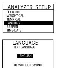
Press the **Setup** button. Using the arrow buttons, select LANGUAGE. Press the **Enter** button.
