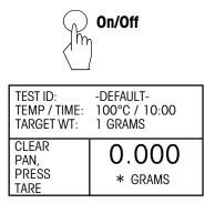
If the display is not visible and the unit is plugged into a power source, press the **On/Off** button.
