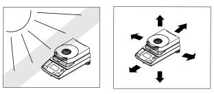
DO NOT install the Moisture Analyzer:
