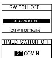
Using the arrow buttons, enter the desired drying time and press the **Enter** button.
