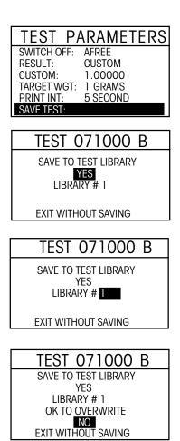
Using the arrow buttons, scroll to SAVE TEST and press the Enter button.
