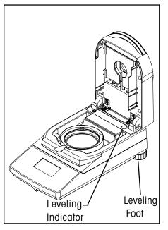
Adjust the leveling feet at the rear of the Moisture Anlyzer until the air bubble in the indicator is centered. The level indicator is located under the cover towards the rear of the Moisture Analyzer.
