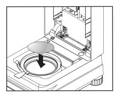
Place the specimen sample in the sample pan (glass fiber pad).
