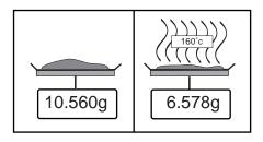
The Ohaus Moisture Analyzer comprises two instruments: a precision balance and a dryer unit. In contrast to other thermogravimetric methods (drying oven, infrared, microwave), the Halogen Moisture Analyzer operates with a halogen dryer unit. This ensures fast heating of the sample and thus guarantees rapid availability of the measurement results.
