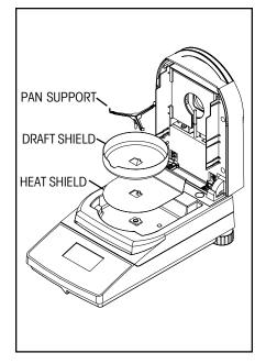
Lift the cover straight up and Install the heat shield in the base of the heating chamber.
