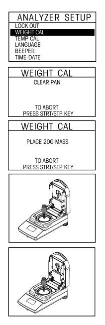
Clear the pan handler, a sample pan should be in place, close the cover on the Moisture Analyzer.
