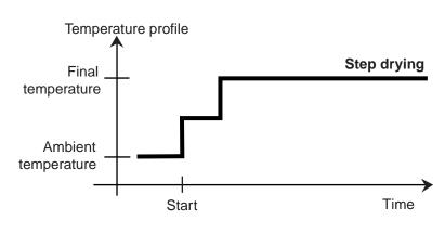
ample, releases only its surface water at 50°C, whereas the water of crystallization can not be separated until 168°C. With this drying program, it is thus possible to determine the surface water and the water of crystallization separately within the same measurement by a controlled temperature profile.
