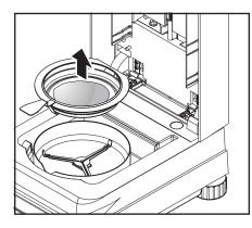
Carefully remove the sample pan handler from the drying area.
