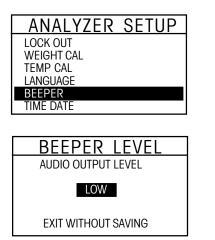
Press the **Setup** button. Using the arrow buttons, scroll to BEEPER. Press the **Enter** button.
