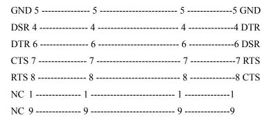
Note: The indicator DB9 female's pin4 and pin6 is shorted, pin7 and pin8 is shorted!
