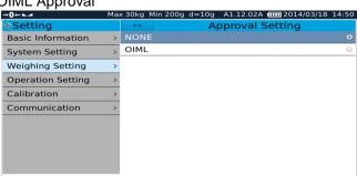
Note: If selected OIML, weighing setting functions can't access.
