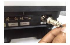
Note: if using 7 wire load cell, please short-circuit SEN+ to EXC+, and SEN- to EXC- for to connect
