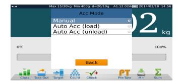
**Auto ACC (load):** When place the goods on the pan, it will accumulate and print automatically once get stable.
