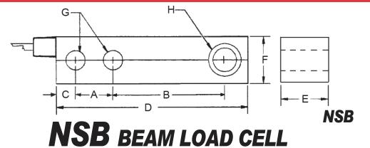
These Shear Beam Load Cells are Interchangeable with Sensortronics 65023 and RTI 5123 (NSB) and Sensortronics 65023-SS and RTI 9123 (NSB-SS). They are constructed from Stainless Steel or Nickel Plated for washability and protection from harsh environments.
