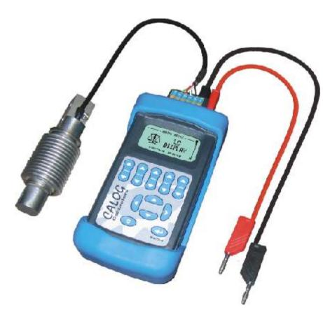
The CALOG - LC II is a portable, multifunction, precision instrument for straingauge loadcell system testing and calibration. This model now includes the powerful ARM processor, a display function (ideal for portable scales or field readings), an SD card for datalogging, a USB port for connection to a computer for certificates or spreadsheets and longer lasting Lithium-Ion battery pack. Supplied complete with carrying case, charger and leads.
