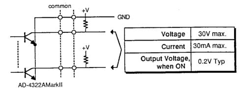
The output circuit is an open-collector type. If you hook-up this line to TTL Logic, please add a pull-up resistor. These pull up resistor may be installed on the option board as there is a space set a side for them.
