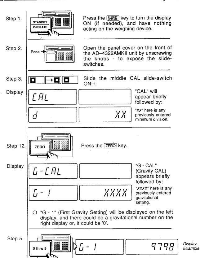
Use the key pad to enter in the gravitational value where the calibration takes place (example: Gravity = 9.798m/s²).
