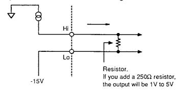
$\Box$  Caution!! This resistor must be high enough for the power consumption. If a  $500\Omega$  resistor is used, power consumption will be:
