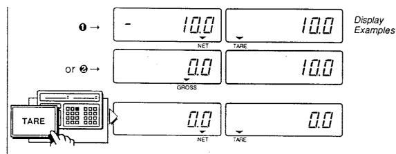
☐ TARE can also be cleared by pressing the TARE key when ① the NET weight display is negative the TARE weight, or ② the GROSS weight display is "zero".
