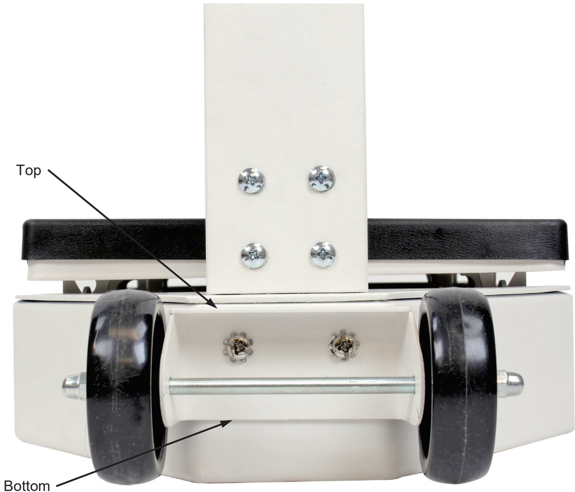
Figure 8. - Attaching wheel assembly to scale base
