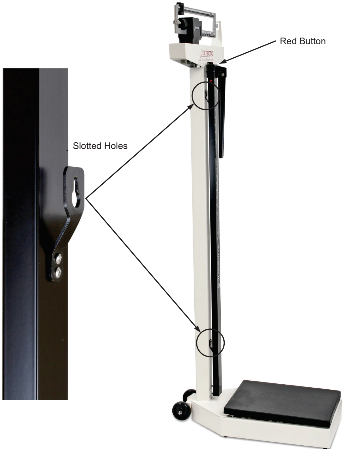
Figure 7. - Place slotted holes in height rod brackets over screws in column
