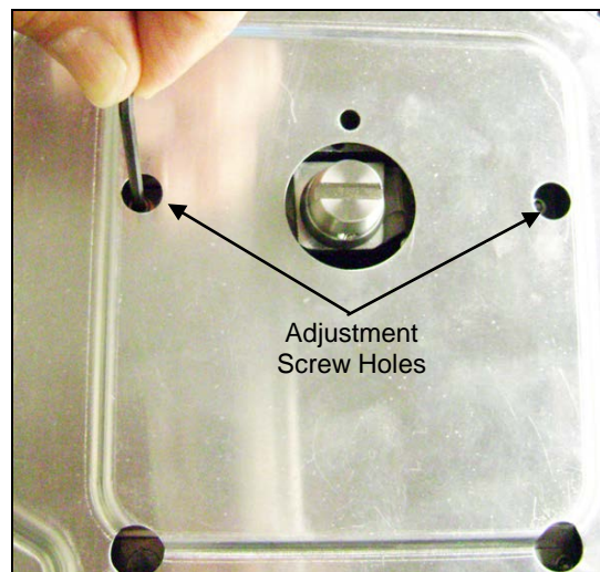
Figure 4-4. Off-Center Load Adjustment screw holes on Adventure Precision models.
