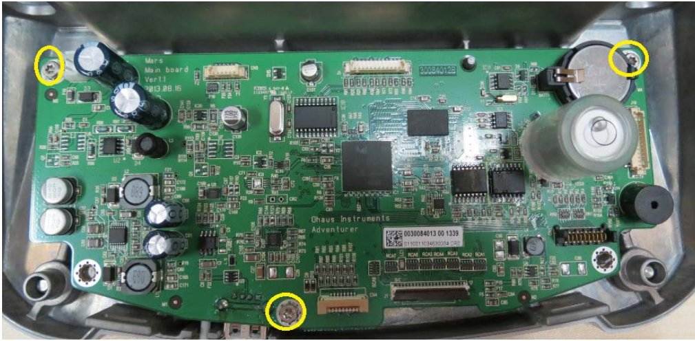
Figure 3-39 Location of the 3 screws securing the Main PCBA to the bottom housing.
