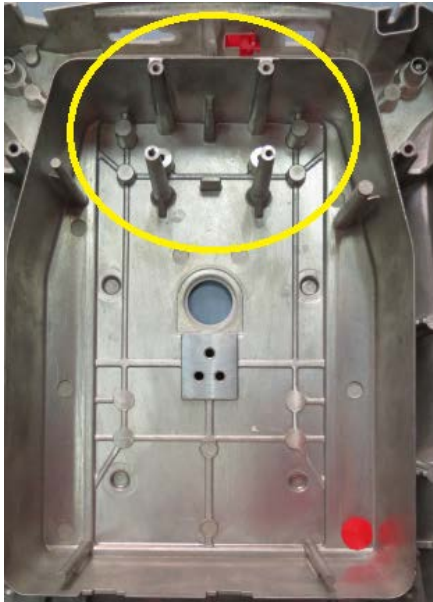
Figure 3-25 Location of the 3 screws holding the load cell to balance bottom housing.
