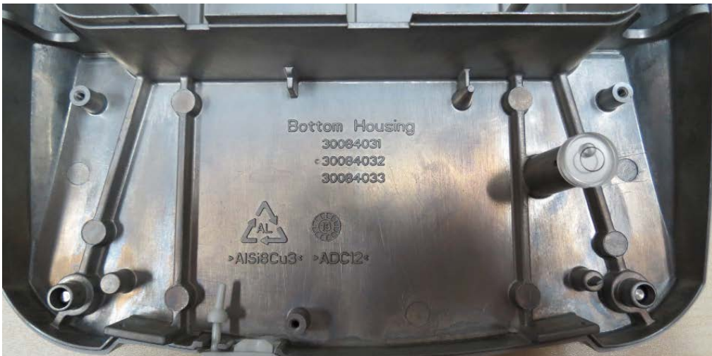
Figure 3-40 Main PCBA removed from bottom housing.
