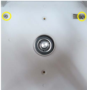
Figure 3-5 Analytical Draft Shield screws location.
