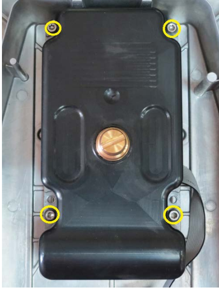
Figure 3-35 Location of the 4 screws securing Strain Gage load cell to the balance bottom housing.
