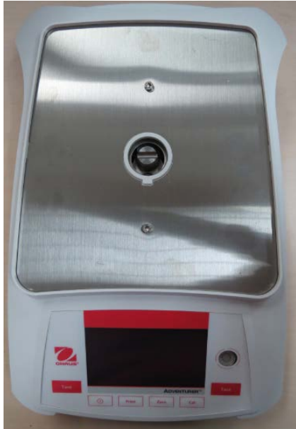
Figure 3-21 Adventurer Precision balance Pan Support removed.
