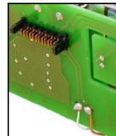
Figure 3-70. Solder points on Position Sensor Board.
