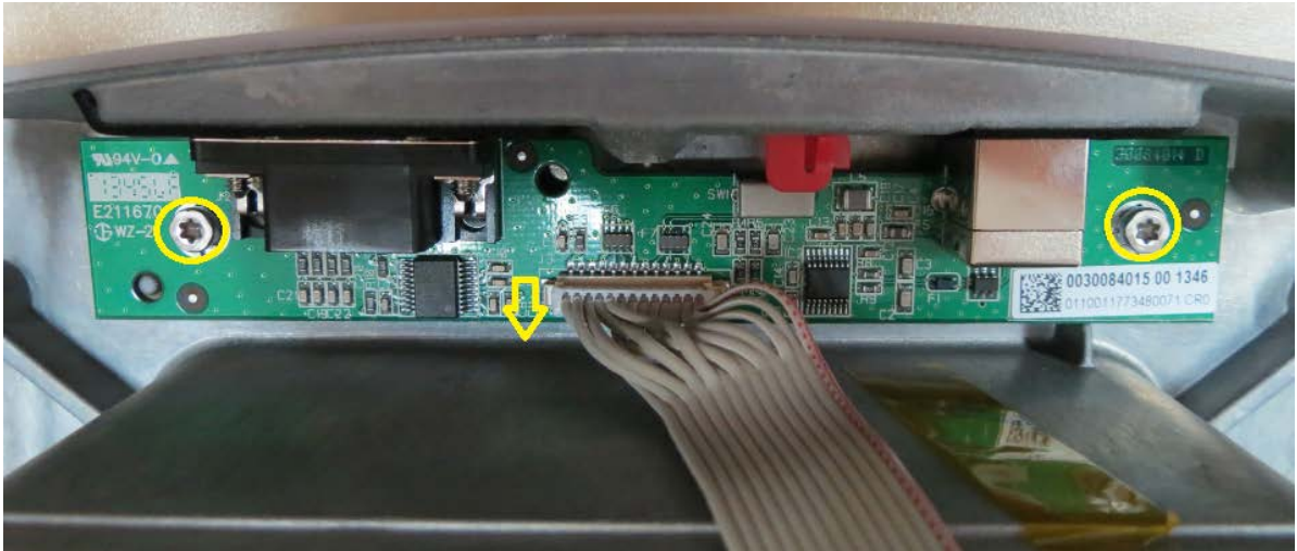
Figure 3-41 Location of the two screws holding the communication PCBA and the cable linking from the communication cable to main PCBA.
