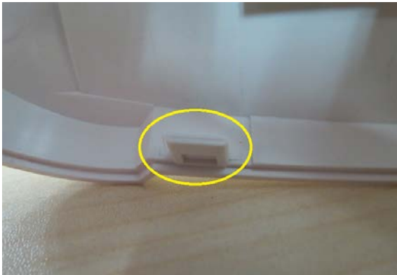
Figure 3-16 Latch located at the right corner side of the top housing.
