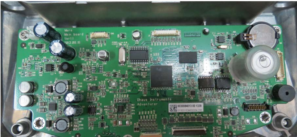
Figure 3-38 Two cables removed from main PCBA.
