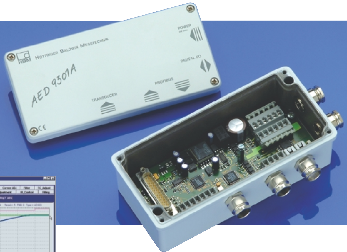
The new AED: compact IP65 housing with intelligent electronics
