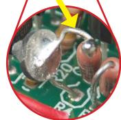
Identify the R4 resistor (brown color), with the thermistor (silver color) soldered to it. The connection between the two components is highlighted with a yellow arrow.
