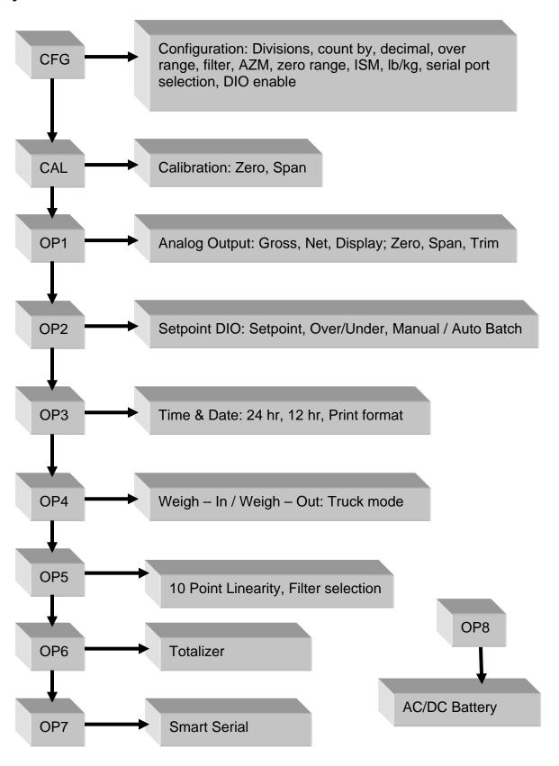
**CONFIGURATION:** "SEL.CFG" Use Gross/Net to enter the menu and step to each category, Tare Recall to select parameters. ENT to return to menu selection.
