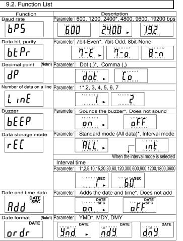
(Note1) Set these functions according to the settings of the personal computer used. \* : Factory setting
