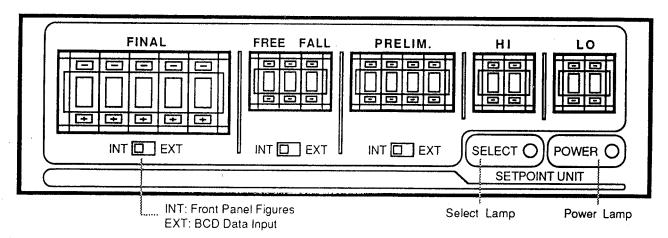
This is an independent unit housed in a separate metal case. It may be directly interfaced to any AD-4323 via attached cable and connector. This option will also accept external input signals - which means that it may be used to control multiple batching operations after receiving external setpoint information.
