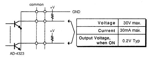
☐ The output circuit is an open-collector type. If you hook-up this line to TTL Logic, please add a pull-up resistor.
