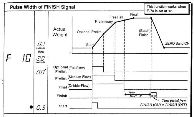
This setting sets the time period from when the FINISH signal is ON to when it goes OFF. *note:* Works only with batching built-in program mode.
