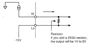
$\Box$  *Caution!!* This resistor must be high enough for the power consumption. If a 500Ω resistor is used, power consumption will be:
