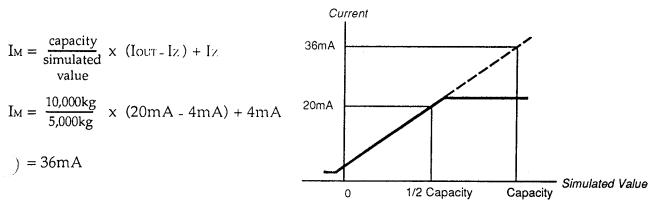
When OUTPUT CURRENT AT FULL SCALE (F-53) is set at 36mA, and OUTPUT CURRENT AT DISPLAY ZERO (F-52) is set at 4mA, then at  $^{1}/_{2}$  capacity (5,000kg) the output current will be 20mA. NOTE: The maximum output will be saturated at 22mA.
