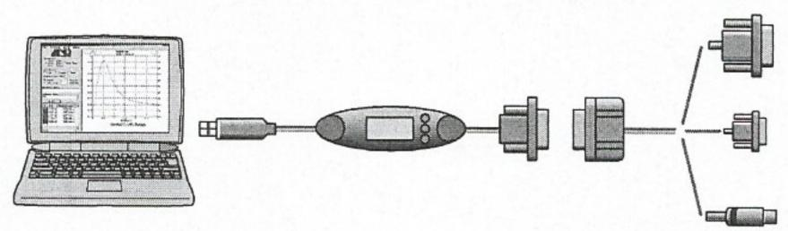
\* Please select either D-Sub 25 pin, D-Sub 9 pin, or DIN depending on your balance/scale.
