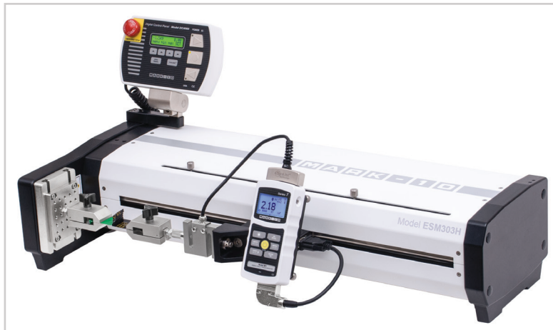
^ ESM303H is shown above configured for a peel test, with a Model M7i indicator, Series R01 load cell, and G1008 film and paper grips.
