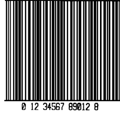
Bar Code L: Interleaved 2 of 5 w/modulo 10 checksum and shipping bearer bars
