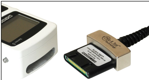
Fig. 3.1 Appropriate orientation of Plug & Test® connector. Sensor model number, serial number, and load capacity may be found on the labels affixed to the connector.
