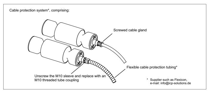
Even without a cable protection system, standard load cells can achieve IP68/IP69K degree of protection. In applications where the PUR cable of the load cell can be chemically or mechanically attacked or destroyed, extra cable protection can be provided by means of standard cable protection systems.
