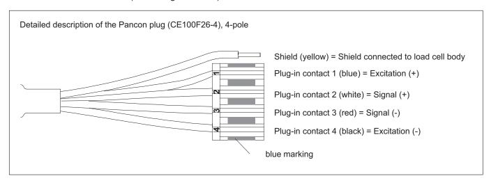
Connection with 6 wire cable, 6 x 0.14 mm<sup>2</sup>/AWG 26 (cable length, selectable: 0.35 m; 1.5 m; 3 m; 6 m)
