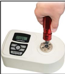
Fig. 1 Gradually exert torque to achieve accurate results
