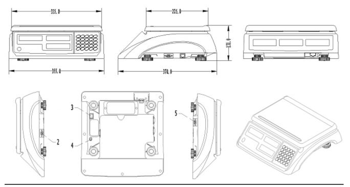
Interface: (2) load cell connector DB9 Male (3) Rocker switch
