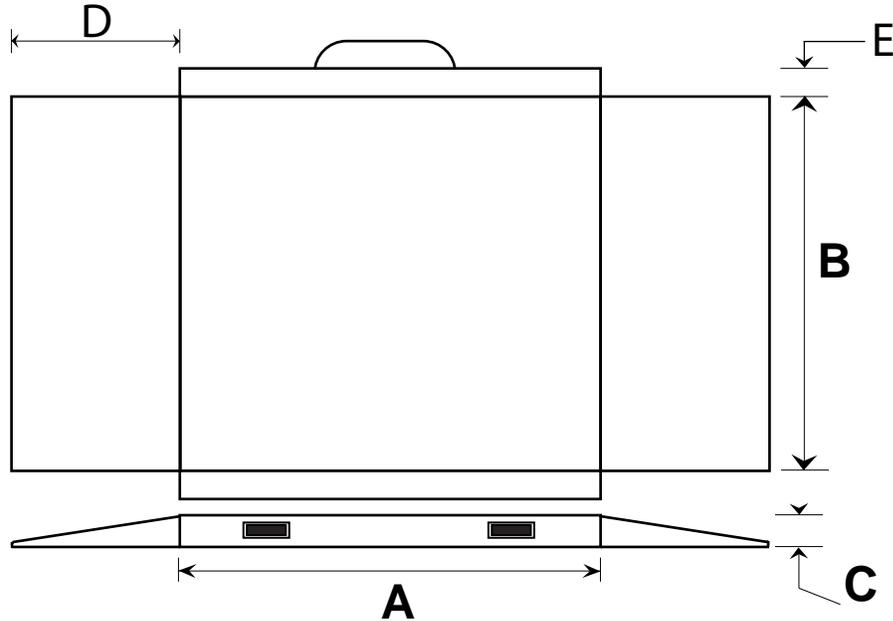
TDB platform is made out of industrial weight heavy duty 1/4" checkered thread steel plate baked powder painted. Two built in folding ramps are low enough to get the hand truck on with ease. Lifting handle and built in wheels for easy moving. Platform uses standard (4) 3 mv/v, 350 ohm load cells and stainless steel signal trim summing junction box. For easy leveling, top bubble level is included. Live rail makes the weighing surface even larger than 36". Adjustable height from 2" to 4.5".
