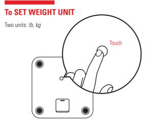
To change the UNIT measurement please touch the round point of the bottom of scale.
