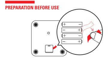
Note: Remove insulating strip beneath the batteries in the battery holder at the back on the scale.
