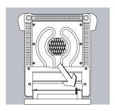
Carefully remove any residue from the temperature sensor
