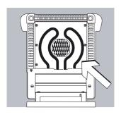
• Use a brush or a damp, lint-free cloth to clean the tubular metal heating element.
