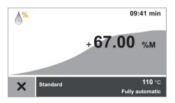
If no target value is set, the measurement process is displayed as a curve diagram.
